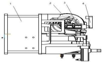
Fig 3 intake manifold clamping mechanism diagram
